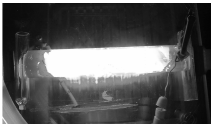
图 4 阳压为 3 400 V 时,真空场发射荧光灯发光图. Fig. 4 Luminescence image of field emission fluorescence lamp with the voltage of 3 400 V
